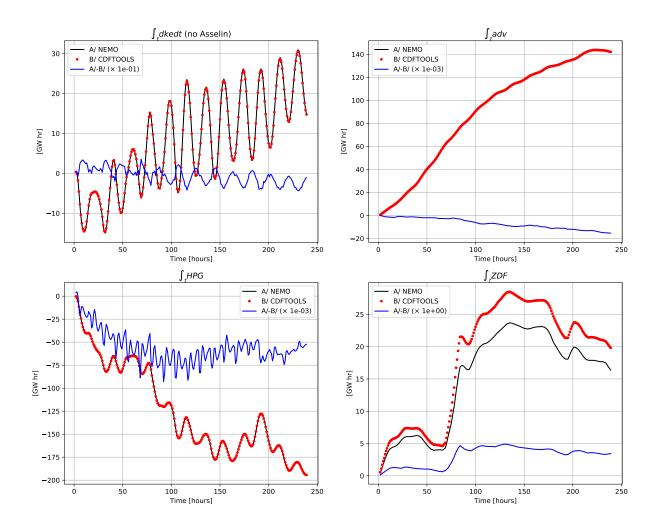
Figure A2. Time integrated KE trends of the full sub-domain, volume integrated time rate of change (upper left), three-dimensional advection (upper right), pressure work (bottom left) and vertical dissipation (bottom right) based on hourly averaged model outputs (black lines), recomputation based on hourly averaged T, S, U, V, W,  $\eta$  (red dots), and the associated errors (blue lines). Note the scale factor used for errors in the legend panels, which differs for each quantities.
