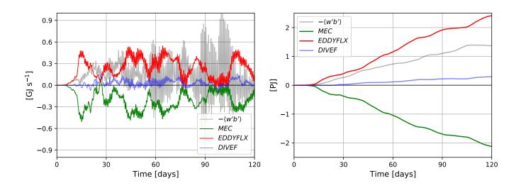
Figure 5. (Left) Time series of volume integrated MEC (green), EDDYFLX (red), DIVEF (light blue) and  $-\langle w'b' \rangle$  (gray) within the green box of Fig. 2, and (right) their time integrated contribution. The 120-day long integrated MEC (EDDYFLX, DIVEF,  $-\langle w'b' \rangle$ ) contribution is -2.12 PJ (+2.41 PJ, +0.30 PJ, +1.38 PJ).
